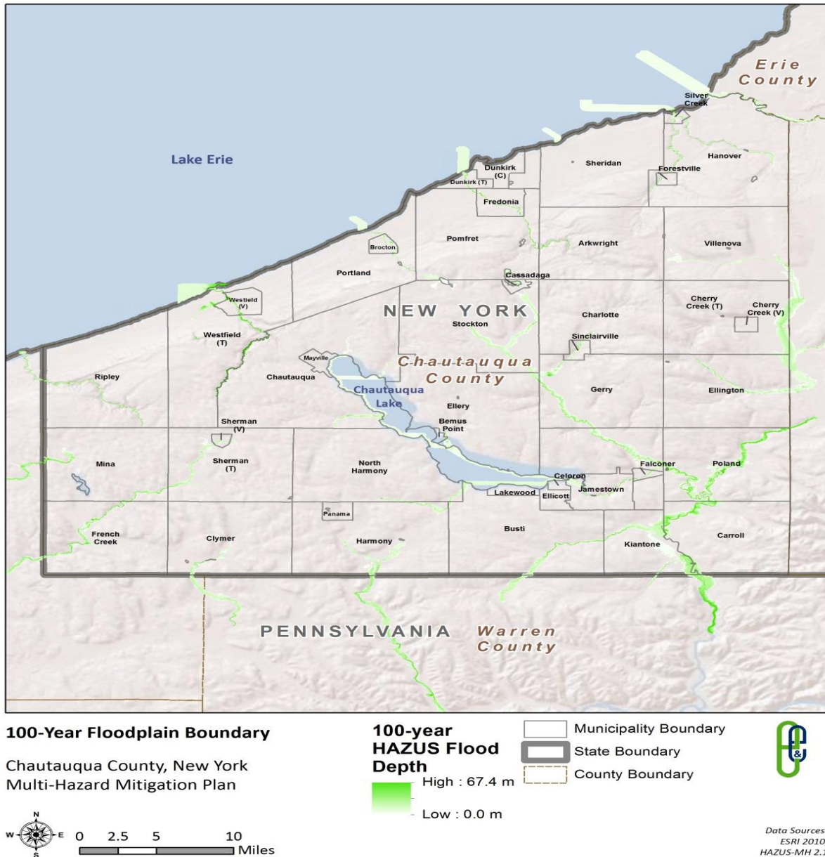
Figure 3-1 HAZUS-generated 100-year Flood Depth, Chautauqua County
